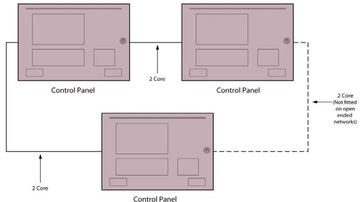
Two core loop wiring ensures network integrity by providing full isolation of faulty wiring segments.
